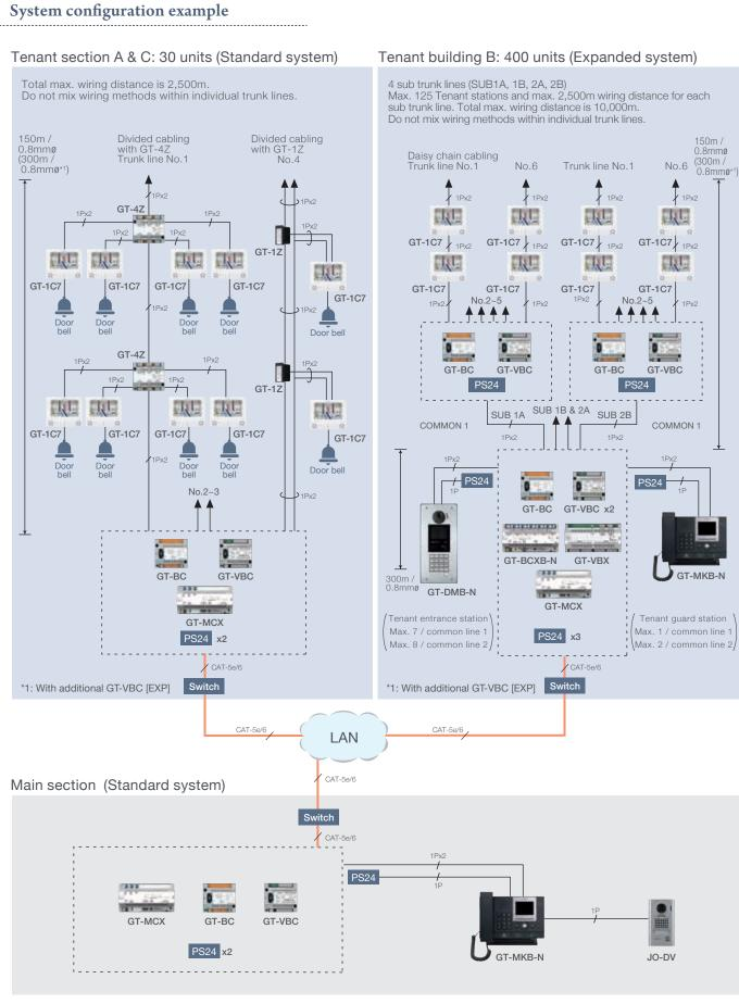
\*Cable: 1Px2, 2-conductor cable solid copper & non-braided, polyethylene insulation.
