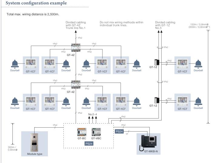
\*Cable: 1Px2, 2-conductor cable solid copper & non-braided, polyethylene insulation.
