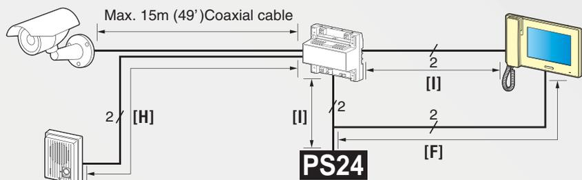
• See "Wiring distance between each device" at left for the maximum distance between each device.
