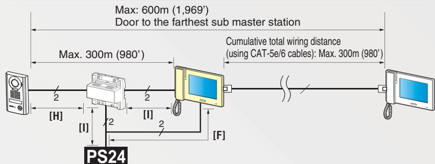
• See "Wiring distance between each device" at left for the maximum distance between each device.
