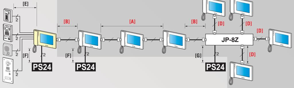
• See "Wiring distance between each device" at left for the maximum distance between each device.
