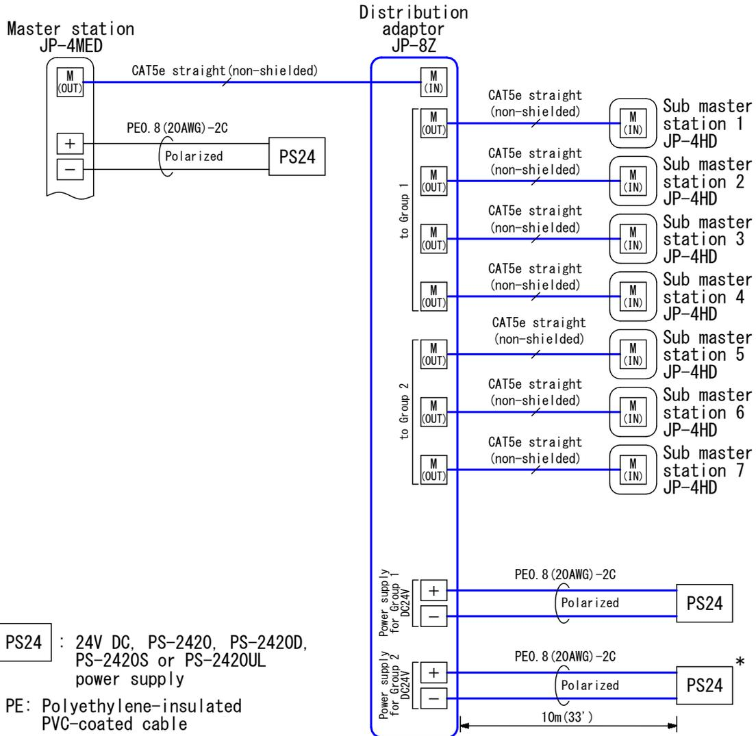
\*. Up to four sub master stations can be supplied with one power supply.
