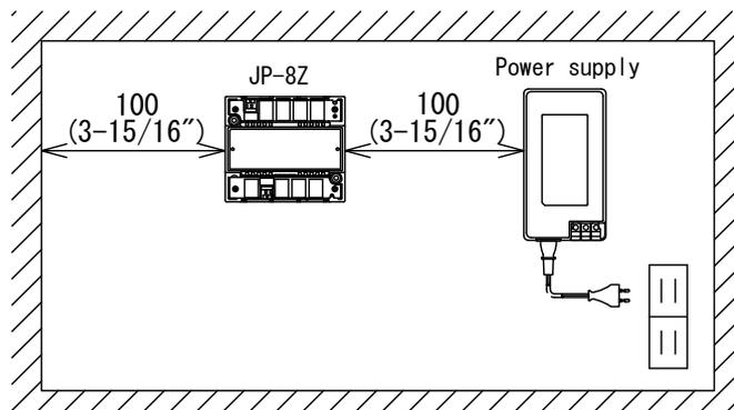
Locate JP-8Z together with Power supply inside an Enclosure box or other protected for limited access.
