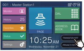
It switches to **[TRANSFER/ON]** and turns orange.
