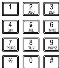
Use the Keypad Buttons to search for a station or zone by number. To search by name, push the LIST Button and use the Camera/Cursor Control and ZOOM/WIDE Buttons to select name search. Once selected, use the Keypad Buttons to type the name of the station or zone.
